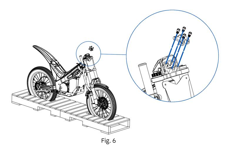
Carefully remove the handlebar, located vertically on the side of the front fork.
