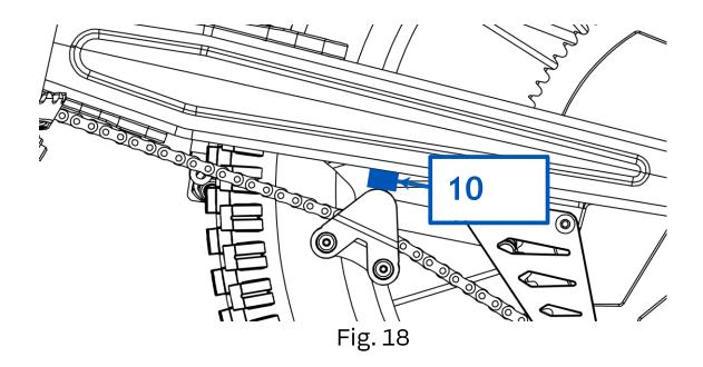
If the chain slack is not within the values indicated above, adjust the chain tension as follows:
