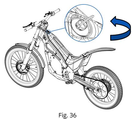
3- Move the cover forward and then you can remove the upper casing of the motorcycle upwards (Figure 37).
