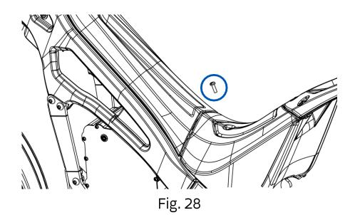
2- Use a flathead screwdriver to pry into the designated slot and remove the cover, which has snap-fit pins secured in the seat holes.
