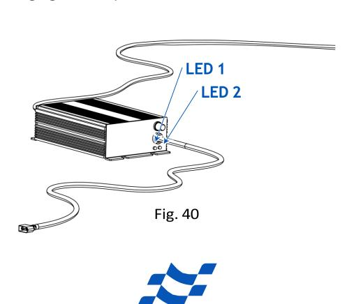
The battery will be fully charged in approximately 2 hours. You will know that the battery is fully charged when the charger's LED 1 is red and LED 2 is green.
