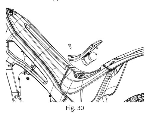
To close the cover, properly align the pins with their mounting holes and secure them by applying pressure. Finally, reinstall and tighten the Allen screw.
