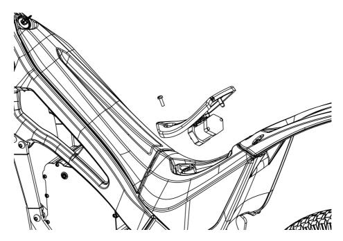
To close the cover, properly align the pins with their mounting holes and secure them by applying pressure. Finally, reinstall and tighten the Allen screw.
