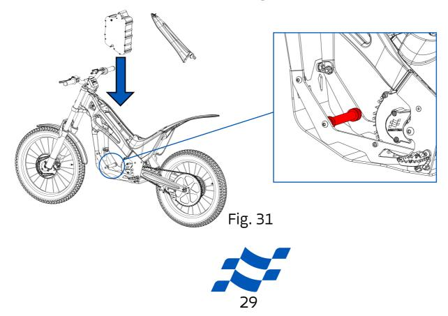
4- Next, attach the battery to the bodywork using the Velcro system.
