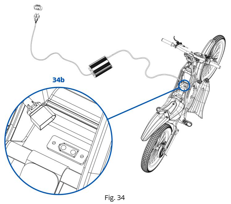
Tthe two LEDs on the battery charger will be red, this means that the battery is charging correctly.
