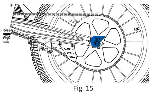
When the chain tension reaches half of the allowed travel, it is necessary to turn the eccentric completely to adjust its position.
