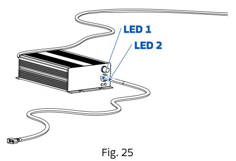
The battery will be fully charged in approximately 2 hours. You will know that the battery is fully charged when LED 1 on the charger is red and LED 2 is green.
