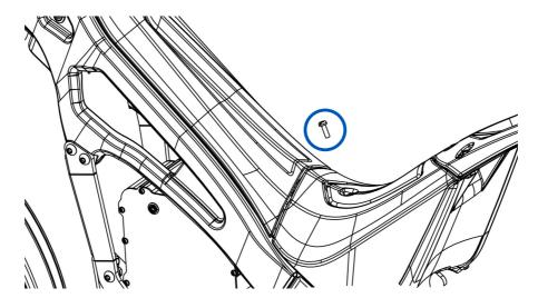
2- Use a flathead screwdriver to pry into the designated slot and remove the cover, which has snap-fit pins secured in the seat holes.
